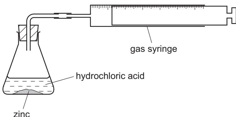
The same mass of zinc was added to different volumes of hydrochloric acid at room temperature, 20 °C. The total volume of hydrogen gas given off in each experiment was measured.
