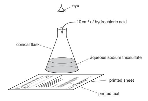
A student used this method to investigate the effect of changing the concentration of the sodium thiosulfate solution on the speed of the reaction.
